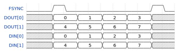
Figure 11: TDM channel numbering
